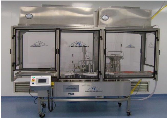
Vial Filler in Class 1000 suite with Class 100 RAB
