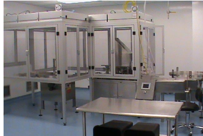
Ophthalmic Filler in Class 1000 suite with Class 100 RAB
