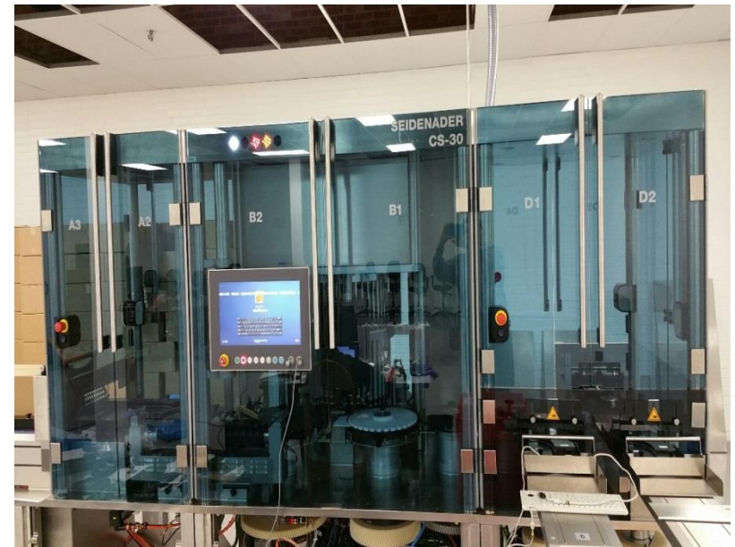
Seidenader High Speed Inspection Machine (400 vials/minute) (being validated)
