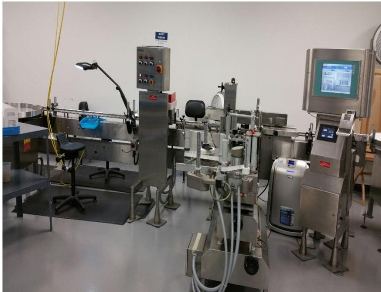
Kalish Labeler with Vision System & Barcode Reader (70 vials/minute)
